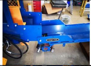
63.) Mount the winch support arm to the processor with the 4 bolts provided.
