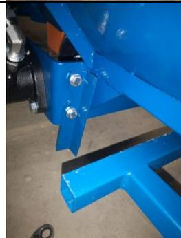
A photo showing the right side guide installed onto the conveyor
