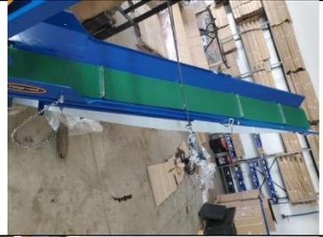
77.) Connect the belt together and put the pin through the lacing.
