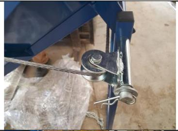
68.) Lift the leg and put lower pin through the leg and tabs to hold it in place.
