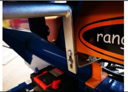
28.) Place large safety cage on the end without any bolts, remove all 10mm nuts & bolts, place blue chainsaw cover on the end of safety cage and line up the bolt holes, tighten all 10mm nut & bolts
