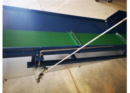
80b) The belt retaining bar is in the travel position in this photo
