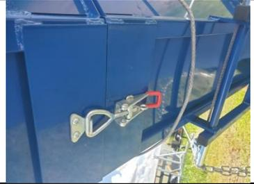
80.) The belt retaining bar shown in this photo that is running along the side of the conveyor is used for retaining the belt when the conveyor is in travel position
