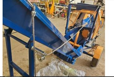
69.) Lower the conveyor and place the second section of the conveyor upside down on the first section.
