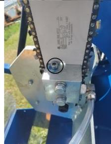
84.) To adjust the chainsaw actuator tab so it will activate valve when moved, make sure that the bolt head and valve rocker line up and the bolt is adjusted to allow chainsaw to engage at the position you want it to.
