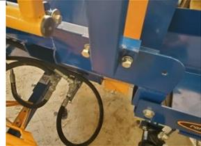
66.) Loosen the winch cable and mount rollers to the pins and put in safety clips
