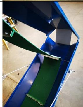
81.) The conveyor is folded up and pinned in the travel position, with the belt retaining bar holding the belt in place
