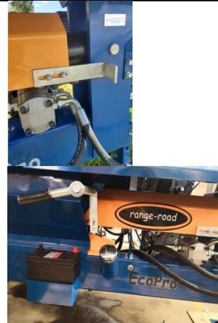
2<sup>nd</sup>) The front bracket hits the post on the manual return arm as the ram returns home, this must hit the post before the ram hits its internal stops, softening the stop.
