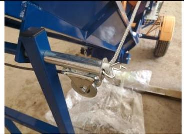
67.) The hook end of the winch cable goes to the loop on the winch support arm.
