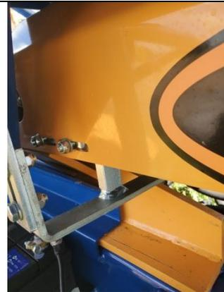
Optional: If the customer is only cutting and splitting shorter lengths, the bar can be reversed to shorten the stroke and reduce the cycle time
