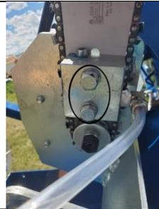
83.) The chain can now be adjusted to ensure the tension is set correctly. Proper chain tension is achieved when the chain can be pulled away from the bar by hand  $\frac{1}{4}$ "...  $\frac{1}{2}$ ". To tighten or loosen the chain, the two bolts can be loosened using a 12mm wrench. Next, the allen key bolt can be turned clockwise to tighten or counter-clockwise to loosen the chain. The two 12mm bolts can be tightened again to hold the bar securely.
