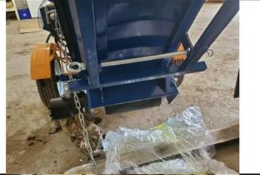
70.) Install bolts and washers at swivel point, remember when tightening the nuts that the conveyor section must be able to swivel, so do not tighten too much.
