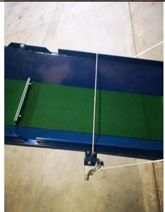
Photo showing the belt being held by the bar as the conveyor is folded
