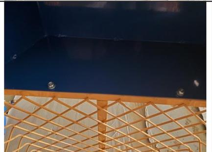
30.) Remove 10mm nut & bolt from safety cage pivot point and remove cotter pin from round bar on safety cage
