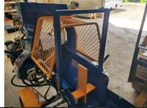
65.) Lift the conveyor section up and line up the holes in the leg with the tab holes and push the long pin through.
