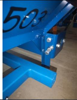
79.) when the conveyor is extended for use the safety clasp should be engaged
