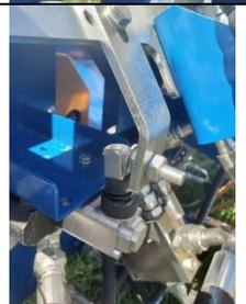
85.) The safety cage by-pass valve must be adjusted so that when the cage is closed the plunger is all the way down with no polished surface showing.
